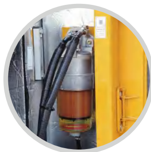
External-mounting fuel filter
